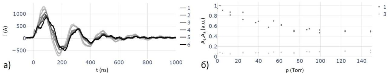
Fig. 1. a) current oscillograms for stationary air at pressure: 1 - 5 Torr, 2 - 25, 3 - 50, 4 - 62, 5 - 99, 6 - 149; b) amplitudes of the main  $A_1$  and third  $A_3$  current harmonics depending on the pressure in stationary air.
