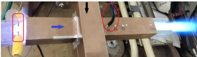
Fig. 1. Photo of propane-air flow ignited by HD. The black arrow is the direction of the incident microwave wave, the blue arrow to the right is the flow direction. The red rectangle highlights the insert with electrodes. The red ellipse indicates the
