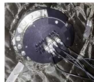
Fig. 1. Si and CdTe detectors for measurements of the fast-scale x-ray perturbations in preliminary experiments in T-15MD tokamak
