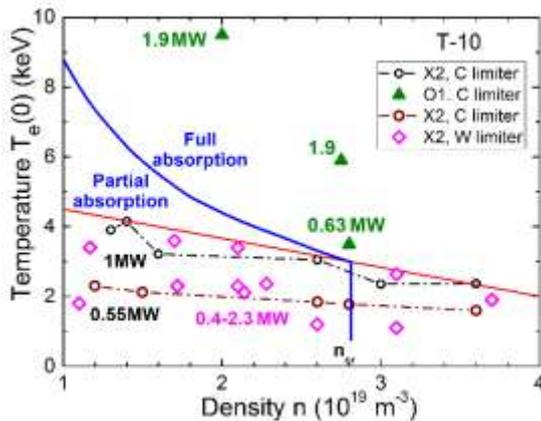
Fig. 1. Comparison of heating at the first (O1) and second (X2) EC harmonics in the T-10 tokamak.
