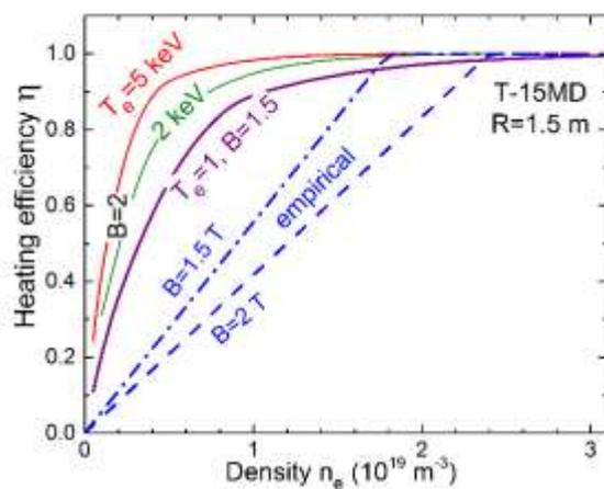
Fig. 2. Theoretical (solid) and empirical (dashed lines) dependences of the of EC heating efficiency in the T-15MD.
